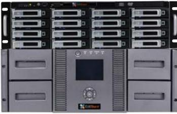
Ark Disk server and 48-slot LTO-6 tape library, for a combination of nearline disk-based and energy-saving tape-based archiving
